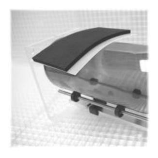
7. You are now ready to make the score. Press firmly on the palm protector while rotating the neck of the bottle. You may rotate the bottle either toward you or away from you. You should hear a slight scratching sound. Be sure to look at the mark you made on the bottle. When that mark comes around to meet the base mark, you have completed the 360 degree score.
