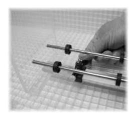
3. Place bottle on the roller carriage and butt the bottom of the bottle against the base. Loosen the Yellow Thumb Screw. Push down lightly on the bottle so that it is resting on the four rubber rollers. This will recompress the Cutting Head so it is just contacting the bottle. Then retighten the Yellow Thumb Screw while you are pressing down.
