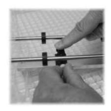
2. Position the glass cutting module by loosening the Black Thumb Screw and sliding the module to the desired location on the Silver Slide Bar.
