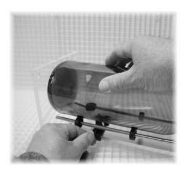
4. You will notice a small Black Line at the top, center, of the base piece. Make a mark on the bottle with a Sharpie Marker. This will be your starting point in line with the base mark. This way you will have a visual indication that you have rotated the bottle 360 degrees. WARNING:
